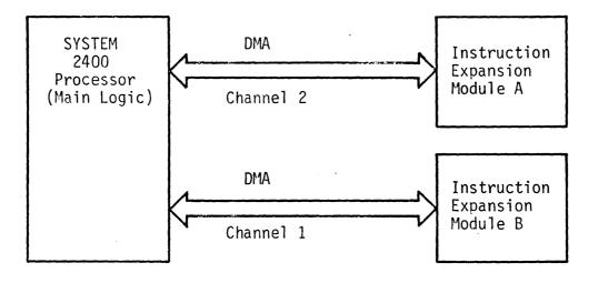
Figure 1-2. Instruction Expansion Modules - Channel Configuration
