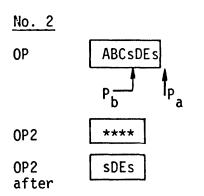
End of buffer operation: EQUAL is set. The pointer is adjusted to one more than the last location in OP1.
