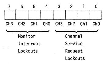
Figure G-2. OTS, ITEM2, Byte 2 Bit Assignments
