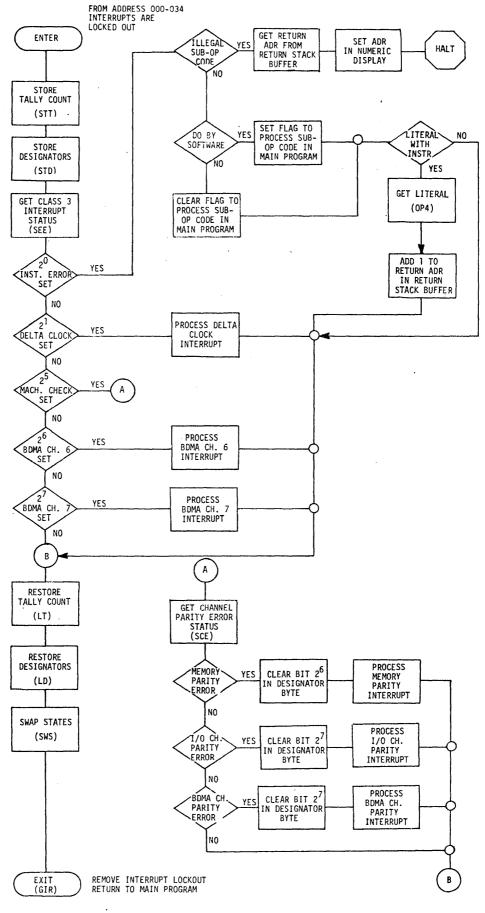
Figure A-5. Special Interrupt Processing Flow Diagram (example). A-11
