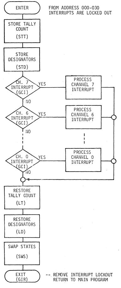
Figure A-4. Service Interrupt Processing Flow Diagram (example).
