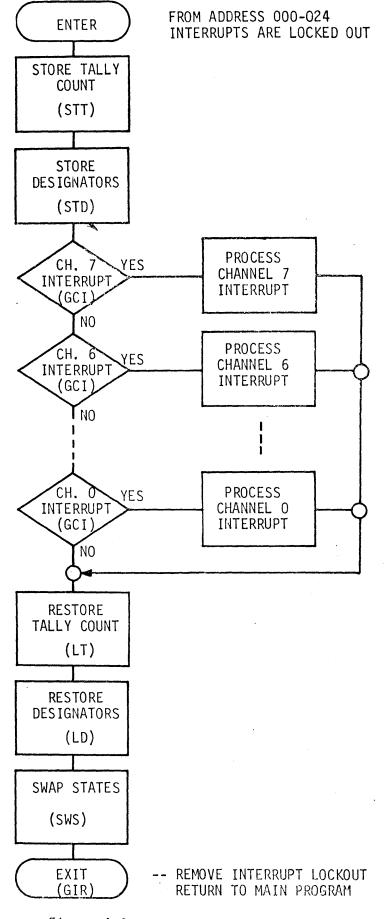
Figure A-3. Monitor Interrupt Processing Flow Diagram (example).
